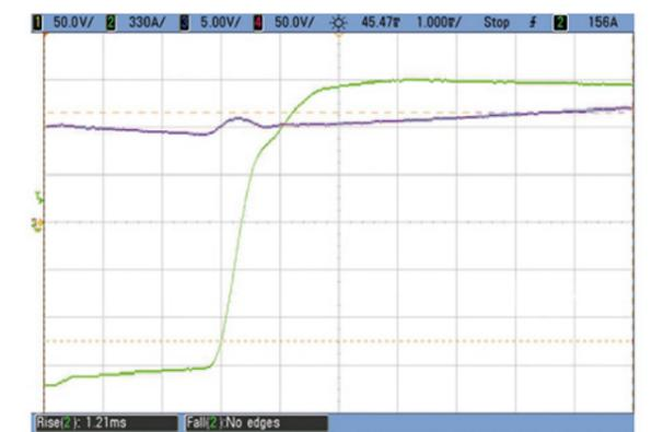
■ output current ■ output voltage
