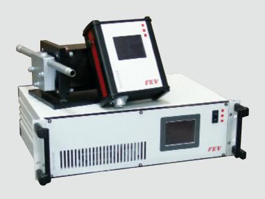
The **FEV ServoCraft** is a universal linear-actuator for operation of throttle valves and injection pumps for combustion engines. The actuator consists of a brushless servo motor. The rotary motion is transformed into a highly accurate linear motion with integrated position feedback signal.
